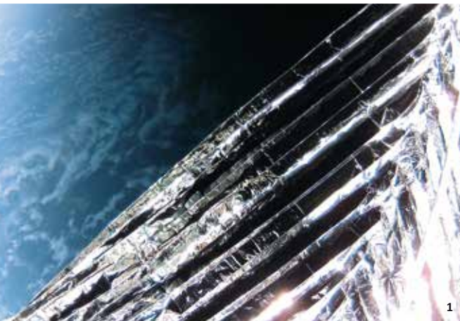
1: In-orbit proof picture of deployed ADEO-N2 onboard ION Satellite Carrier of D-Orbit (Source: HPS, Dec. 2022)
