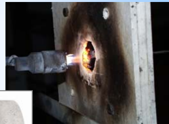
Heat Test with secondary protection up to 1600°C
