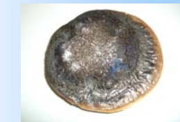
Heat Test with secondary protection up to 1600°C
