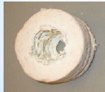
Insulation and protection after arc jet test
