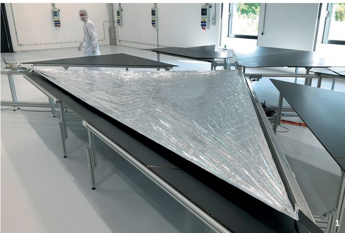
1: Section of ADEO-L Engineering Model (deployment testing on ground)
