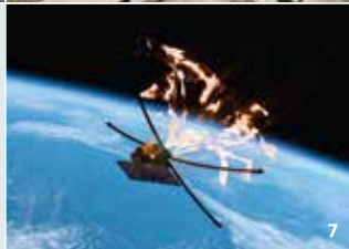
6: ADEO-L Engineering Model (deployment test on ground) 7: Animation of 25 m 2 ADEO-L with a 0.8 m x 0.6 m x 1.2 m satellite with a satellite mass of 300 kg during atmospheric entry
