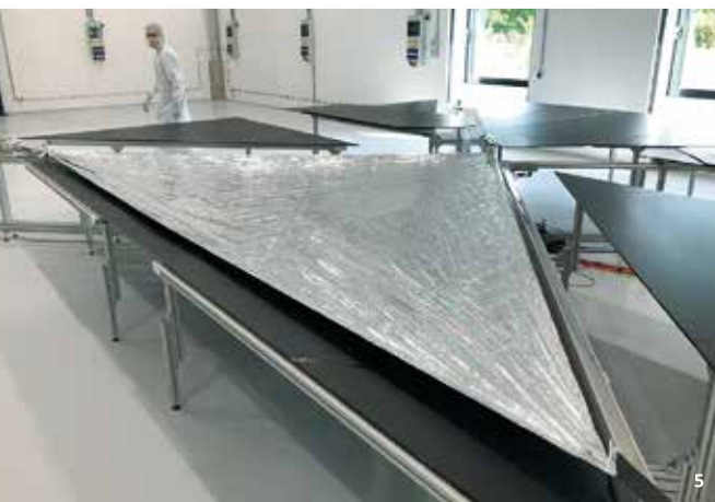
5: Section of ADEO-L Engineering Model (deployment testing on ground at DLR-Bremen)
