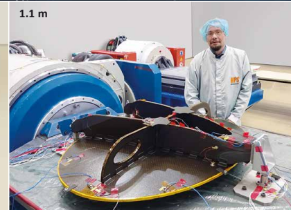
1.1 m Ka-Band reflector EQM for German Heinrich Hertz mission under vibration test
