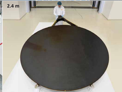
2.4 m Side deployable reflector Q/V-band in full CFRP design tested under qualification level
